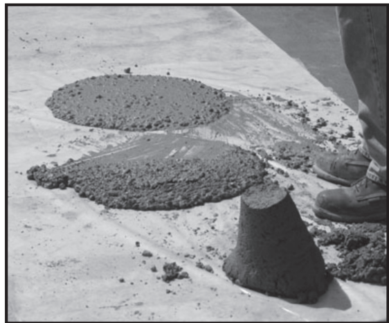
FIGURE 6 Regular slump shown in a cone and SCC concrete shown in a puddle or flow
